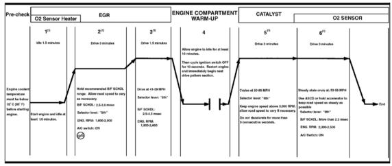
(i) Indicates this drive pattern section must be repeated, without turning the ignition off, if it is interrupted by releasing the accelerator when not directed to do so.
