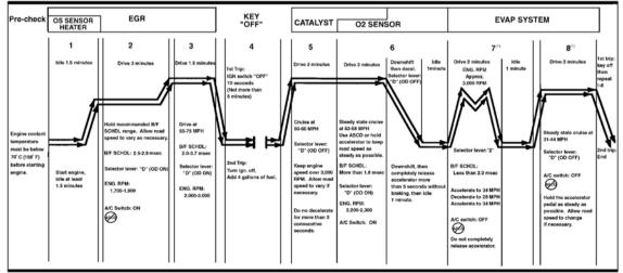
NOTE: It is better to perform this driving test when fuel level is less than 1/2. If fuel level is greater than 1/2 more time may be required to complete EVAP sections of the drive of
