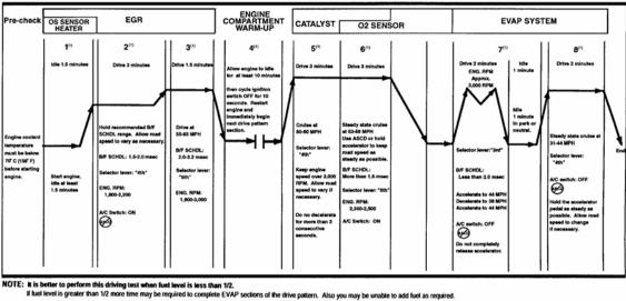
Indicates this drive pattern section must be repeated, without turning the ignition off, if it is interrupted by releasing the accelerator when not directed to do so.
